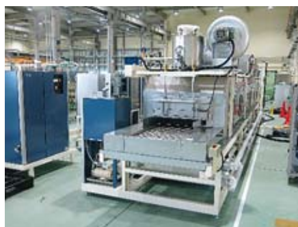
Net conveyor type shower washing system
