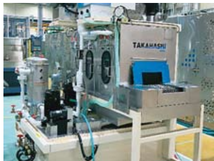
Net conveyor type shower washing system
