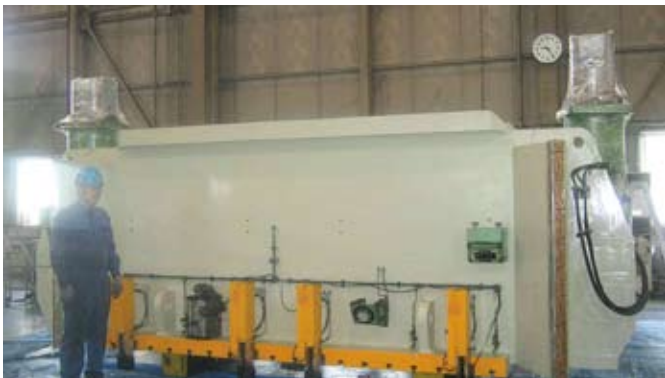
New slide Length 6m, weight 25t
