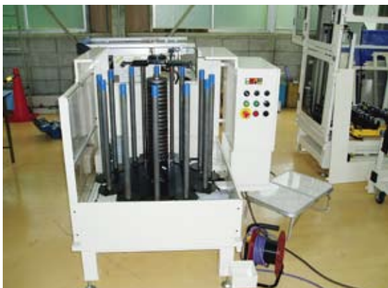
Skewer type rotary stocker
