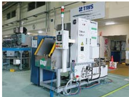
Batch type shower transfer system
