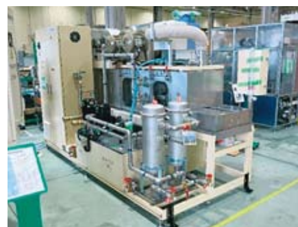
Net conveyor type shower washing system
