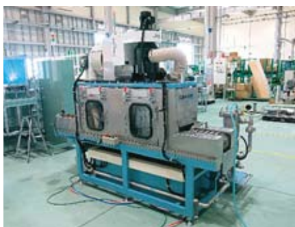
Net conveyor type shower washing system
