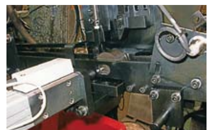
Width thickness Poka-Yoke system (Monosashi-Kun)
