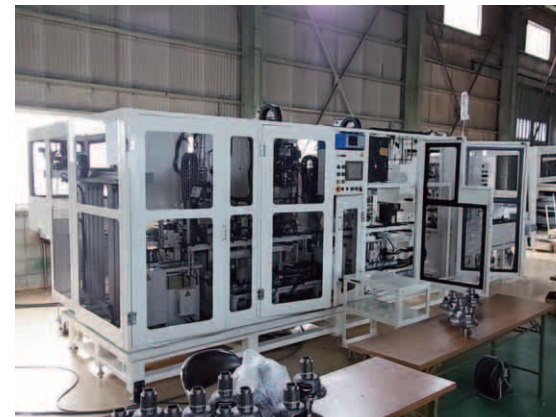
Differential ASSY - Clearance inspection device
