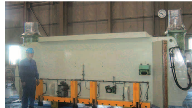
New slide Length 6m, weight 25t
