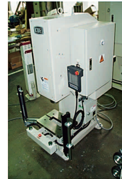
Electric servo press 5 TON KSV-5
