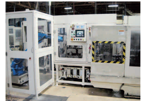
Balance shaft - Gear/pin press-fit machine
