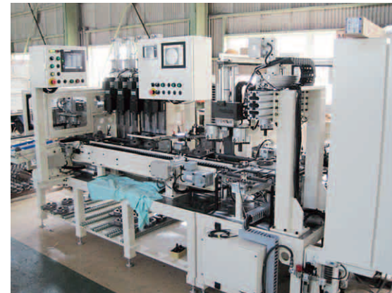
Differential side gear - Final inspection device
