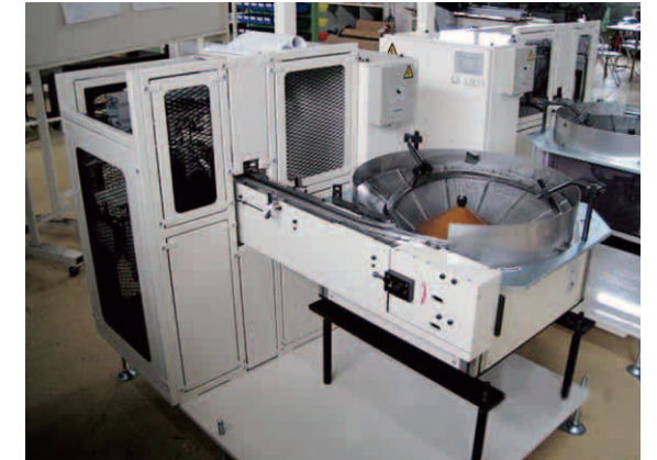
Original ball feeder - Material feeder
