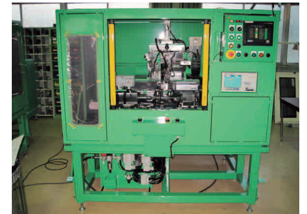
Pulley shaft - Deflection measuring instrument
