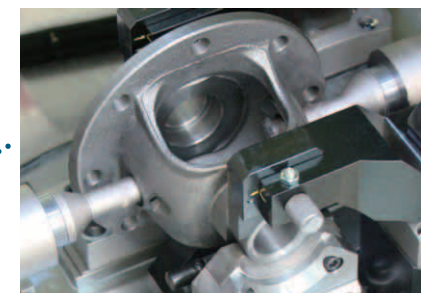
Shaft hole drilling (left/right) Simultaneously tap hole drilling, semi-finishing, and opening chamfering Ultra-high speed finishing with high-speed reamer
