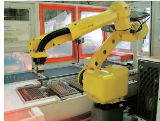
Articulated robot - Palletizing system
