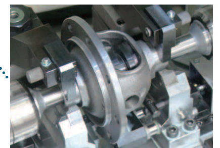
End processing (left-right) High speed machining with vertical cutter
