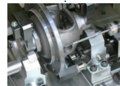
Knock hole drilling Semi-circular face machining with milling Spot facing with end mill Knock hole drilling
