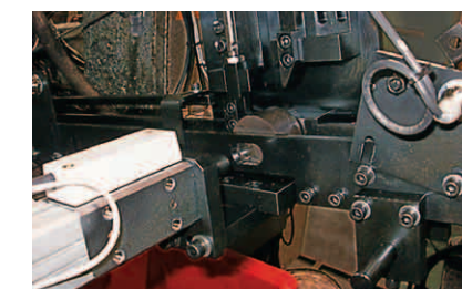
Width thickness Poka-Yoke system (Monosashi-Kun)
