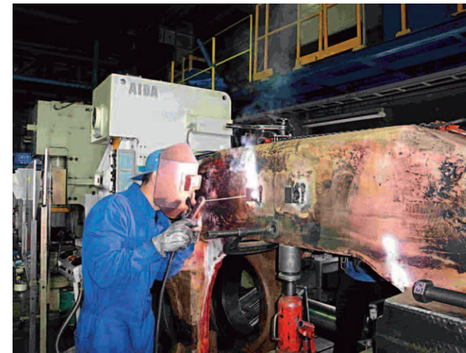
Welding and repairing 1600t slide damage
