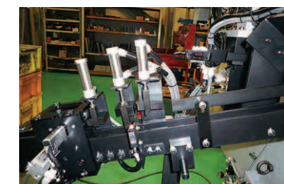
Total length Poka-Yoke system (GT sensor)
