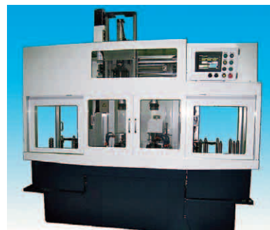
2-head type chamfering machine (with loader)
