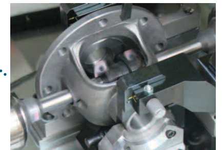
Spherical face drilling (left-right) Machine the spherical face and chamfer the inner face
